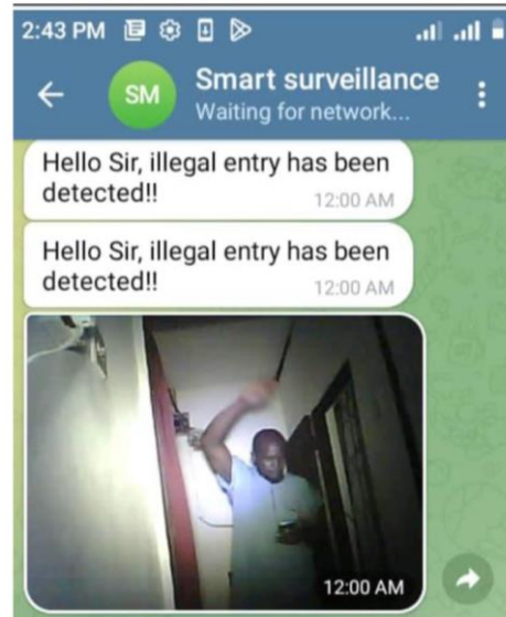
Figure 4. Sample photo snapshot and messaging system log sent via Telegram.
