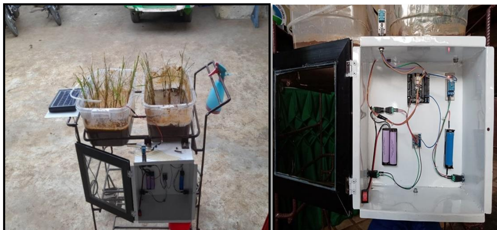
Figure 3. Hardware System in Steel Container Frame with the sample Rice Plant
