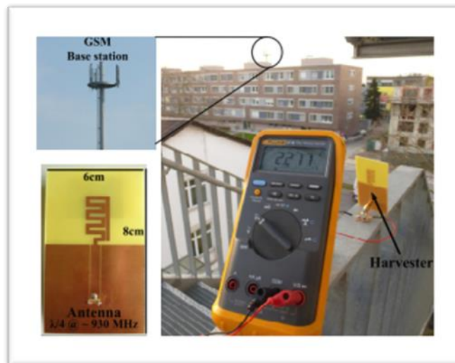
Figure 2. Setup for Measuring the Voltage from a Cell Site source and the RF Harvester Got a Measured Average Voltage of 2.3 Volts
