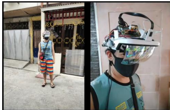
Figure 4. The Wearable Smart Face Shield (SFS) Prototype
