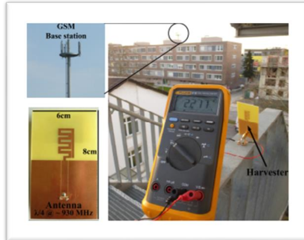
Figure 2. Setup for Measuring the Voltage from a Cell Site source and the RF Harvester Got a Measured Average Voltage of 2.3 Volts (from Nimo et al., 2015)
