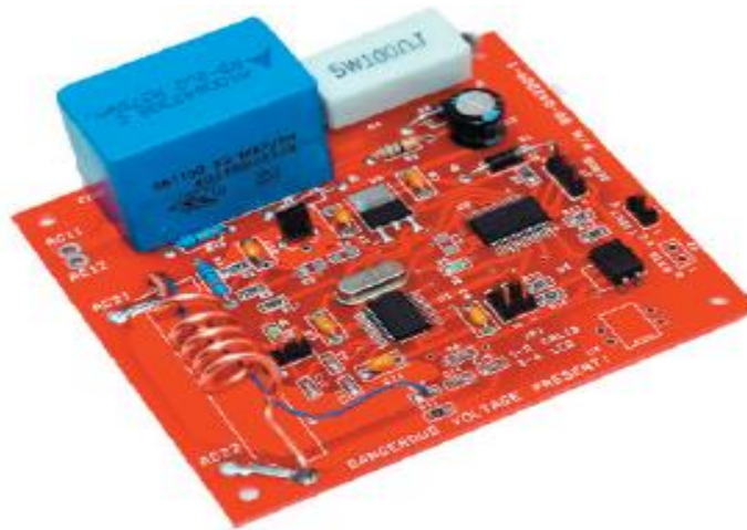
Figure 4. AC Power Analyzer
