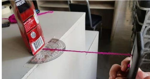
Figure 7. Front Angle Barcode Testing
